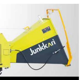
↑ The HJ-250 G model is a chipper with a hydraulic feeding device. Its two feed rollers are powered by the tractor's hydraulics. The HJ-250 GT model is almost identical to it: the only difference is that its feeding device has an independent hydraulic tank and pump. This means that no additional hydraulics is needed.
