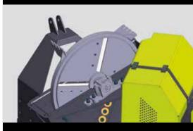
↑ The HJ-170 chipper has four blades that can be adjusted continuously depending on the desired woodchip size. The blow wings will finalise the woodchips and blow the chips effectively to the desired location through an adjustable discharge chute.
