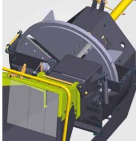
The discs of the HJ-250 and HJ-261 model come with four blades you can adjust continuously depending on the desired woodchip size. The blow wings will finalise the woodchips and blow the chips effectively to the desired location through an adjustable discharge chute.
