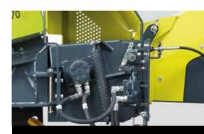
↑ In the picture you can see a hydraulic feeding device of HJ-170 G. It has one feed roller powered by the tractor's hydraulics. The handle is used to control the rotation of the feed roller.
